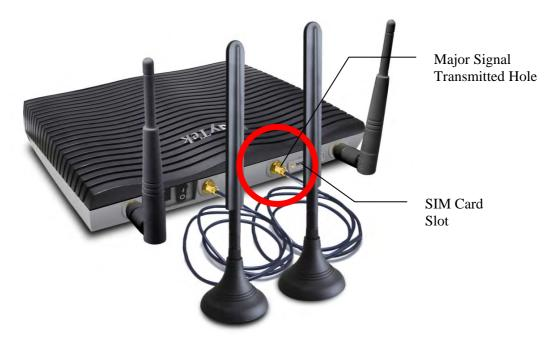
Note, if only one antenna shall be installed, please use the mounting hole (major signal transmitted hole) near to the SIM card slot.
